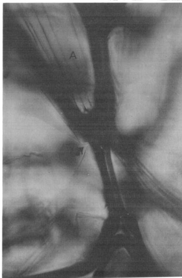
Figure 12 Photograph of cell deformed at crack tip of a foam of density 35 \text{ kg/m}^3
